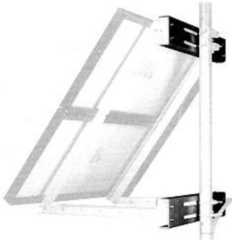
**OPTION:** For easy installation of the SP-100 Series Solar Panels to the side of a pole or mast, racks are available for all models of panels. Complete hardware for assembly and for tipping the panels to the same angle as the sun (perpendicular) comes with this option. Once the panels are installed on the rack, they can be tipped from 0° to 90° of the ground. Two each two inch u-bolts are provided for securing the rack to a fixed location. To order, add suffix -R to model number.
