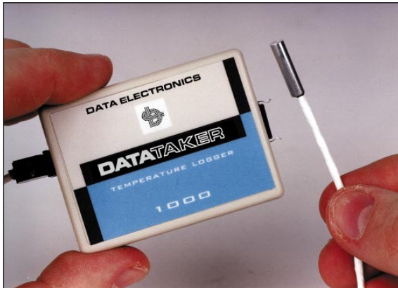
Datataker 1000 Two input channels — one for on-board ambient temperature plus one for optional remote temperature probe
