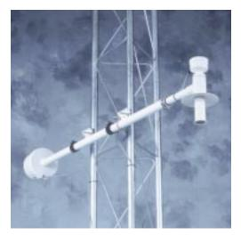
improve aspiration efficiency. Specially selected plastic materials provide high reflectivity, low conductivity, and maximum weatherability.
